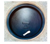
**INSTALLATION:** No special tools are required to install PARSON MANHOLE INSERTS. Just remove the manhole cover and clean the rim of the frame. Place the PARSON MANHOLE INSERT on the manhole frame rim and replace the manhole cover.
